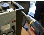
3.6 Slide side cover back about half way off until tab in side cover lines up with slot in cooler frame.
