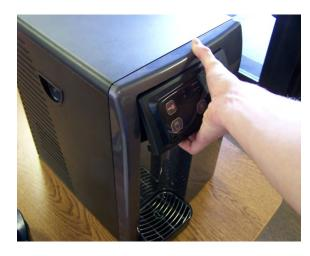
6.2 Remove circuit board cover, by removing (2) screws from the back and pulling the cover off.
