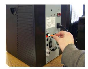
2.2 Connect tubing to feed connector on back of cooler.
