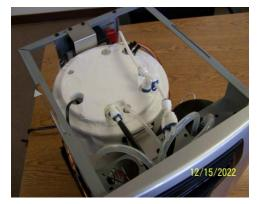
4.2 Disconnect and emove tubing from both sides of 'T' fitting
