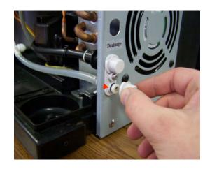
5.3 Remove (4) electrical connectors from hot tank temperature sensors.
