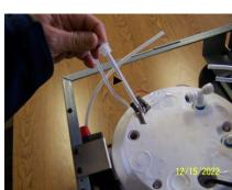
4.7 Remove ice bath level sensor probes (3).
