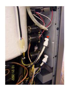
7.4 Remove 3 quick connect fittings from the 3 outlet ports of the 3 solenoids
