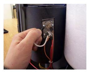
5.4 Remove (2) electrical connectors from hot tank heater coil leads.
