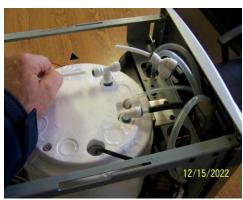
4.3 Remove silicon tube and 1/4" tube from fitting
