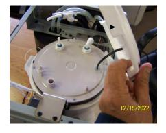
4.10 Remove 4 screws securing top/Purechill assembly
